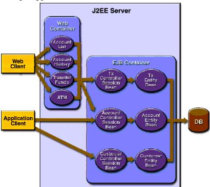
This diagram illustrates a 4/5-tiered architecture: client / web-server / application logic / business logic / persistence. The J2EE server includes both a web container and an EJB container. Client applications are both standalone and browser-based. Transactions are controlled by session beans; interactions with core business data is via entity beans.
